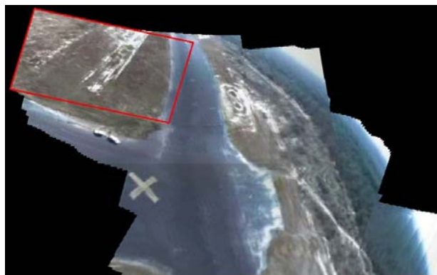
Figure 1: Sample mosaic from MAV stabilization system, with the current image frame outlined in red.
