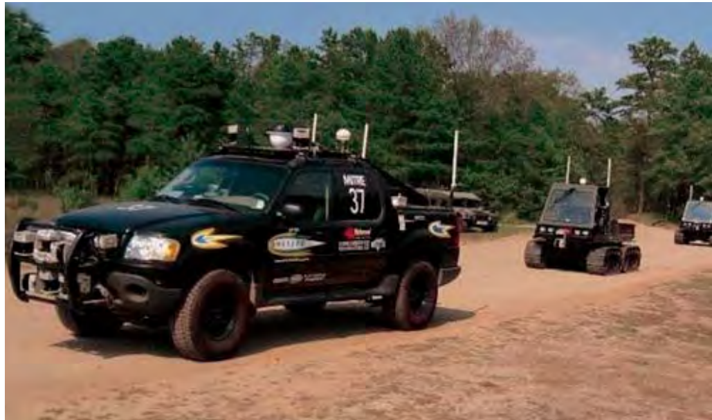
The MITRE Meteor, a 2004 Ford Explorer Sport Trac, leads two tracked Centaur vehicles in a leader-follower experiment at Ft. Dix, Trenton, NJ.
