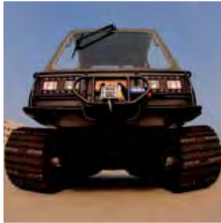
Two driverless Centaur vehicles like this one were the followers in a leader-follower experiment at Ft. Dix, Trenton, NJ.
