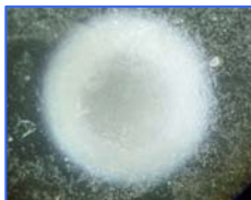
Bubbles of CO 2 gas are visible on film surfaces.
