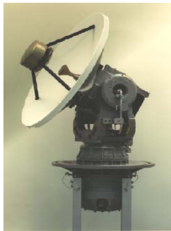
Airborne Command Post EHF Antenna: 30" High
