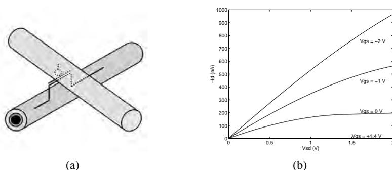
Figure 3: Illustrations of (a) a crossed-nanowire p-channel field effect transistor (PFET) and (b) a model of the I-V characteristic for this device. The experimental basis for this model was obtained from Huang *et al.* [7]. For this transistor, the threshold voltage, at which the device produces essentially zero current and turns “off,” is observed to be approximately +1.4 V.
