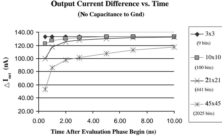
Figure 11: Plot of  $\Delta I_{out}$  versus time.  $T=0$  corresponds to the beginning of the evaluation phase. The time it takes for  $\Delta I_{out}$  to reach its maximum value has implications on the speed of the memory. The simulations above have zero capacitance between the nanowires and the substrate.
