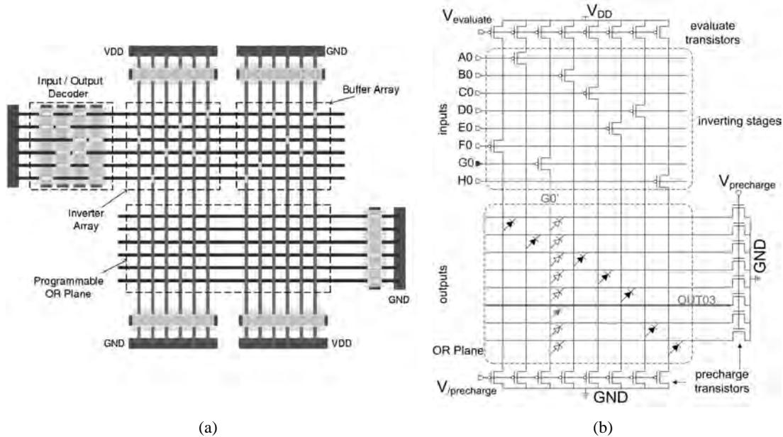
Figure 18: Illustrations of (a) the DeHon-Wilson PLA Architecture and (b) an  $8 \times 8$  inverting block. The eight vertical wires shown in part (b) correspond approximately to the vertical wires in the left-hand side of the subarray in part (a).
