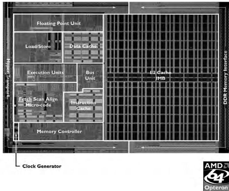
Figure 16: AMD Opteron™ die photo with annotated block structure [125].
