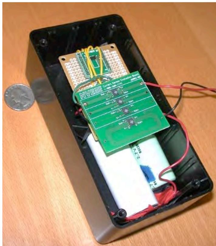
**Figure 6.** Initial laboratory prototype of nanotechnology-enabled portable power system that was assembled and tested in this work. A better packaged version of the system, with the control circuit breadboard replaced by an integrated circuit chip, would occupy only about  $60 \text{ cm}^3$ .
