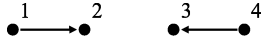
Fig. 3. Example failure scenario of BTPS. Node 1 has HP packets intended for Node 2. Node 4 has LP packets intended for Node 3. The four nodes can only hear their adjacent neighbors' transmissions. If Node 4 gains access first then it can suppress the HP stream from Node 1. As part of Node 4's contention, Node 3 sends a CTS that mutes Node 2. When Node 1 contends, Node 2 cannot respond. Node 1 considers the contention a failure, increases its contention window and contends again. The busy tone scheme cannot affect Node 4 and so Node 1 can only seize the channel if by chance its contention window expires between Node 4's transmissions.
