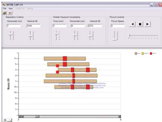
The CAP-CV Interface allows users to “dial in” specific parameters to highlight potential conflicts.
