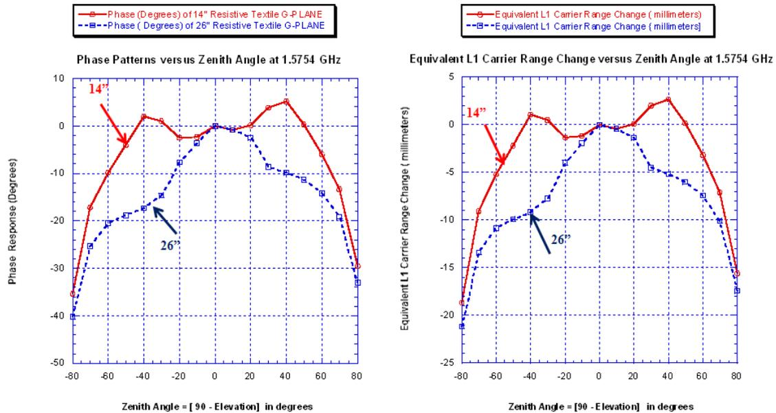
**Figure 12. Phase Response & Equivalent Range Change versus Zenith Angle = 90° – Elevation Angle at 1.5754 GHz for 26" and 14" Square Resistivity Tapered Ground Planes**
