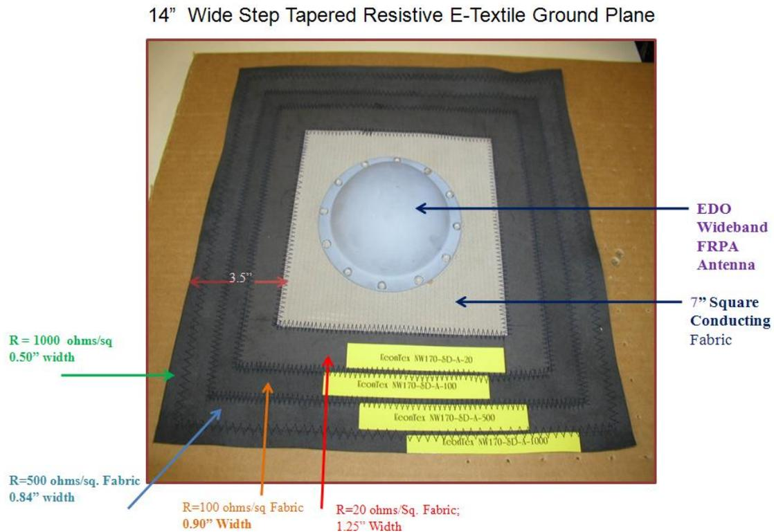
**Figure 8. Picture of the 14" Square E-textile Ground Plane with Step Resistivity Tapering**
