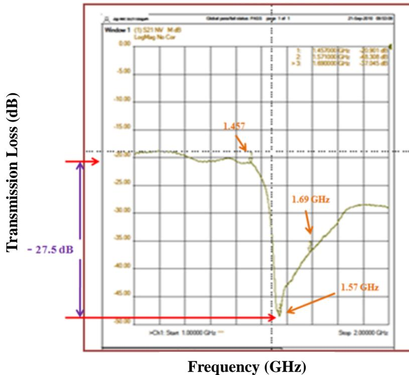
**Figure 15. Measured Attenuation versus Frequency of TM Type Surface Waves on a Metal Surface by the EBG Ground Plane versus Frequency; the Band Gap Starts at 1.57 GHz**
