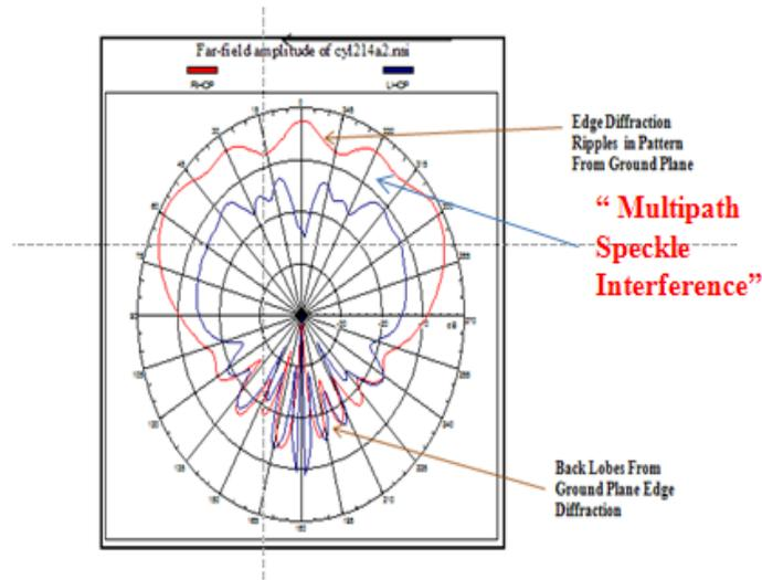
**Figure 1(b). Measured Pattern of a Patch Antenna on Metal Ground Plane**
