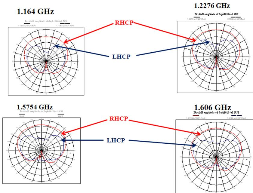
**Figure 7. Measured Elevation Plane Patterns of the 26" Resistivity Tapered E-textile Ground Plane at Four Different Frequencies Covering the Entire GNSS Band**
