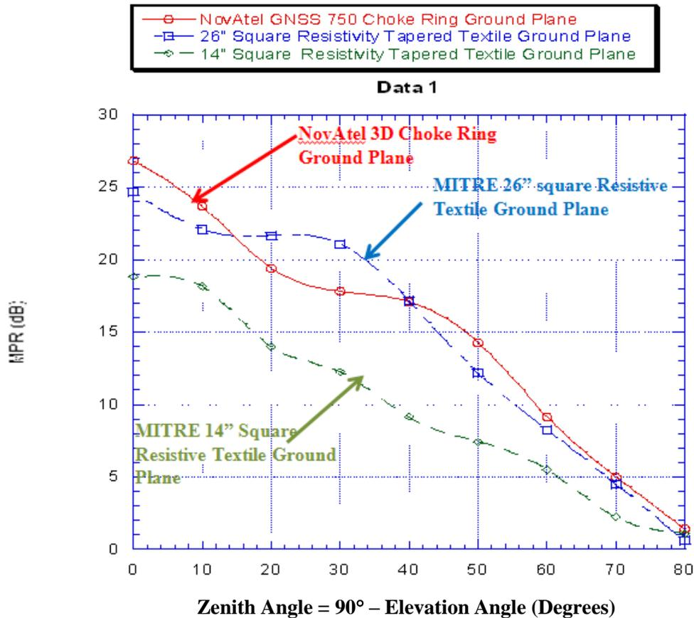
**Figure 11. Comparison of Measured Multipath Ratio (MPR) as a Function of Zenith Angle = 90° - Elevation Angle at 1.5754 GHz for Three Different Ground Planes**
