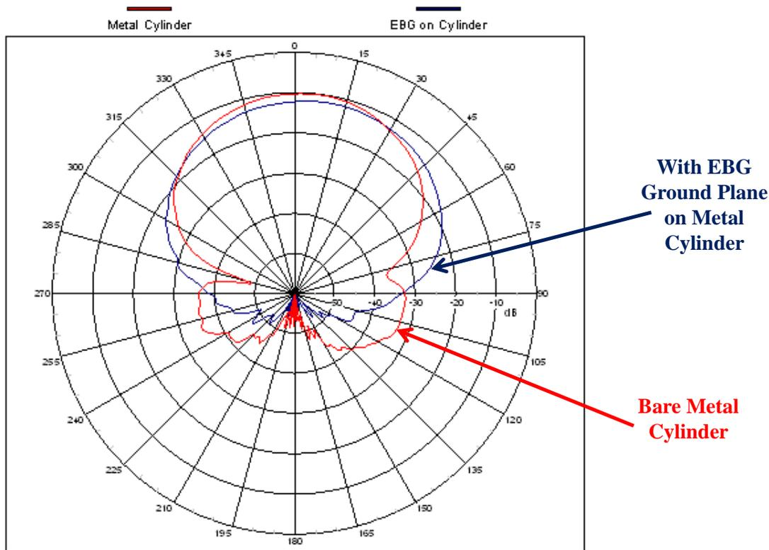
**Figure 19. Comparison of the Measured Roll Plane RHCP Radiation Patterns of the RSW Textile Antenna Placed on the Bare Metal Cylinder and on the EBG Ground Plane placed on the Metal Cylinder**
