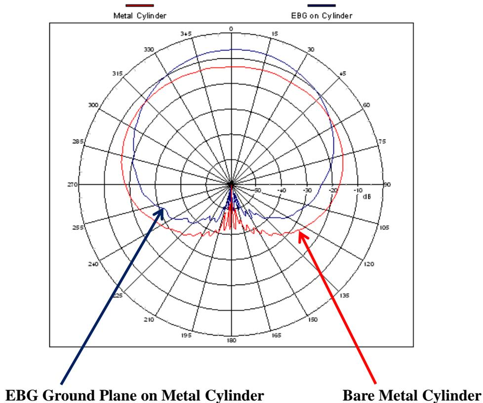
**Figure 17. Comparison of the Measured RHCP Roll Plane Patterns of an EDO Antenna Measured on 5' Diameter Bare Metal Cylinder and with EBG Ground Plane on the Cylinder**
