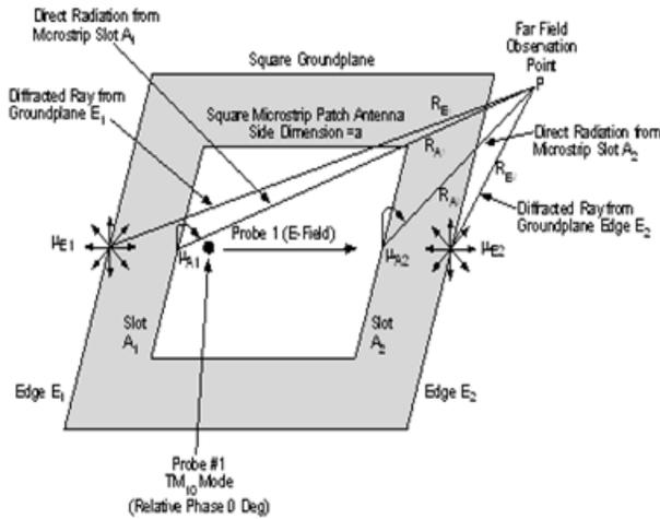
**Figure 1(a). Edge Diffraction Effects from a Metal Ground Plane on the Radiation Pattern of a Patch Antenna**
