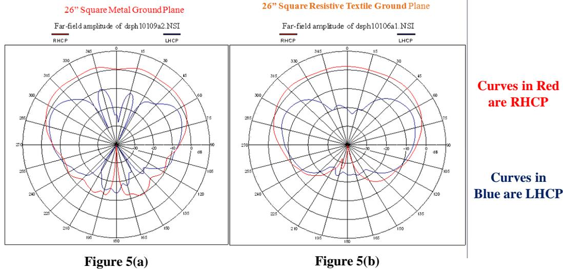
**Figure 5. Comparison of Measured Elevation Plane Patterns of the EDO Antenna on 26" Square Planar Metal Ground Plane [shown in Figure 5(a)] and the 26" Square Textile Ground Plane with Exponential Resistivity Tapering [shown in Figure 5(b)]**
