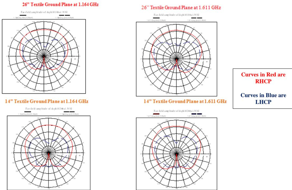
**Figure 9. Comparison of the Measured Elevation Plane Patterns of the 26" and 14" E-textile Ground Planes at 1.164 GHz and 1.611 GHz**
