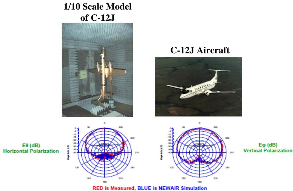
**Figure 3. Scale Model Measurement of the Effects of Diffraction from the Curved Surface of the Fuselage on the Radiation Pattern of a Patch Antenna on a C-12J Aircraft [From Reference 1]**
