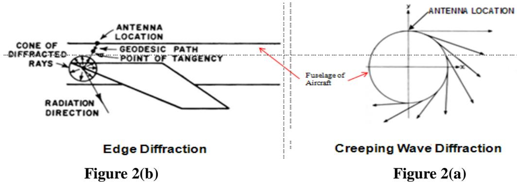
**Figure 2. Curved Surface (“Creeping Wave”) Diffraction and Edge Diffraction Effects from GNSS Antenna on Top of Aircraft**
