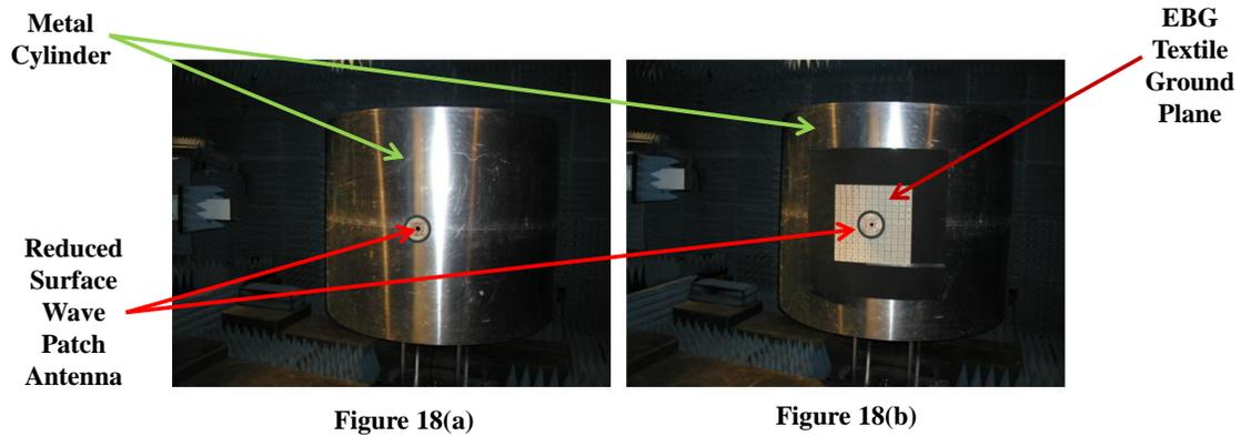
**Figure 18. Reduced Surface Wave (RSW) Microstrip Shorted Annular Ring Antenna Placed on the Large Metal Cylinder – without the EBG Ground Plane [shown in Figure 18(a)] and with the EBG Ground Plane [shown in Figure 18(b)]**
