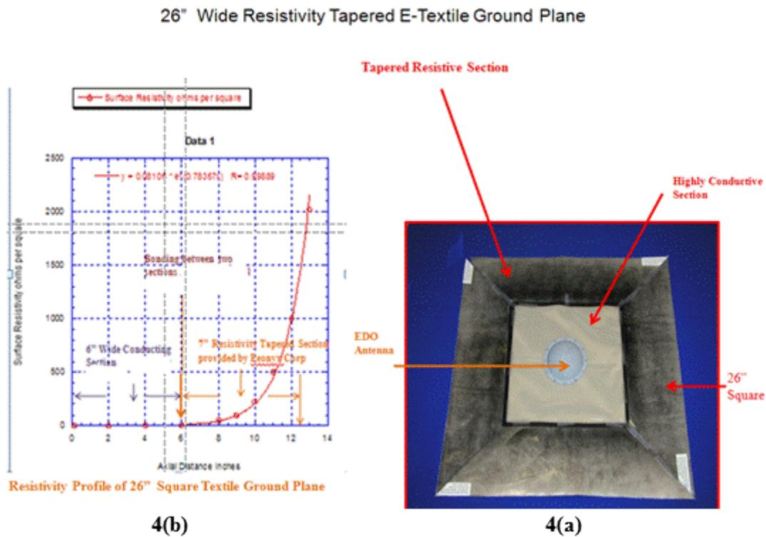
**Figure 4. E-textile Ground Plane with Exponentially Tapered Resistivity**
