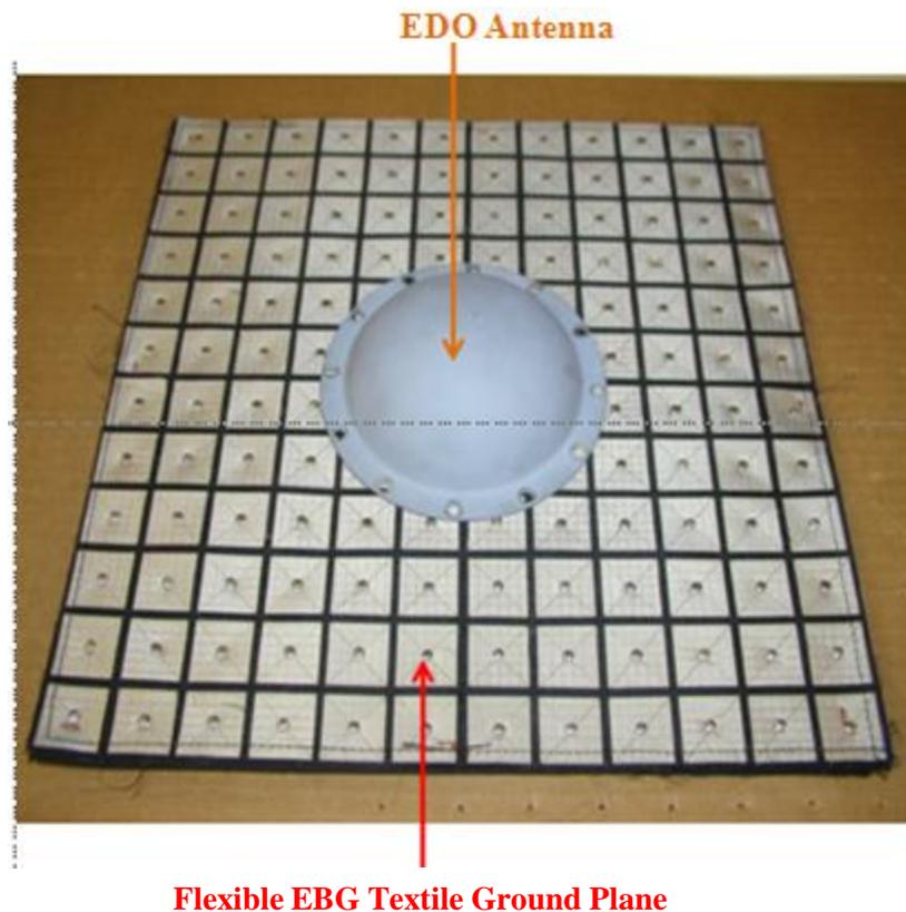
**Figure 13. Flexible “Electronic Band Gap (EBG)” Ground Plane for Suppression of Curved Surface Diffraction from GPS Antennas on Aircraft**
