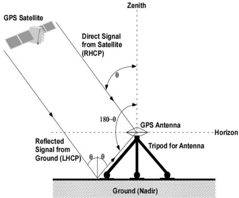
**Figure 10. Diagram Illustrating Multipath Reflected Signals Received by a GNSS Antenna**
