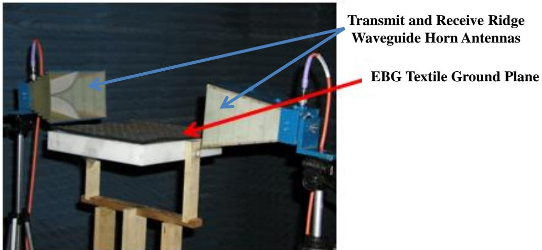
**Figure 14. Measurement of the Surface Wave Frequency Band Gap of the Electronic Band Gap (EBG) Textile Ground Plane**
