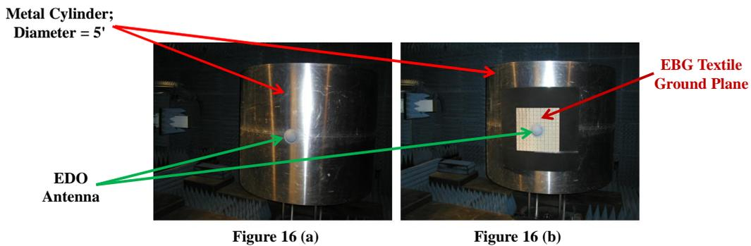
**Figure16. EDO Antenna Placed on the Bare Metal Cylinder [Figure 16(a)] and on the Metal Cylinder Covered by the EBG Ground Plane [Figure 16(b)] to Verify Suppression of Antenna Backlobes**
