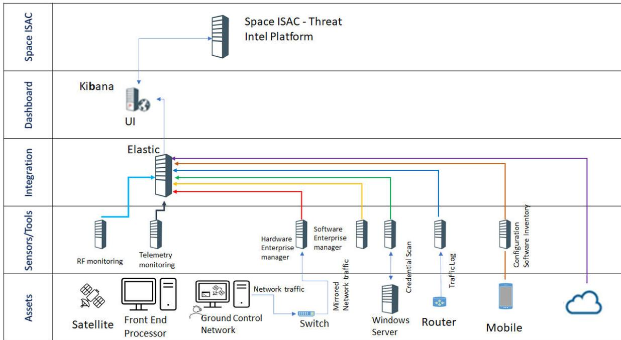
**Fig. 1 Monitoring Architecture for Notional Space Operator Organization**
