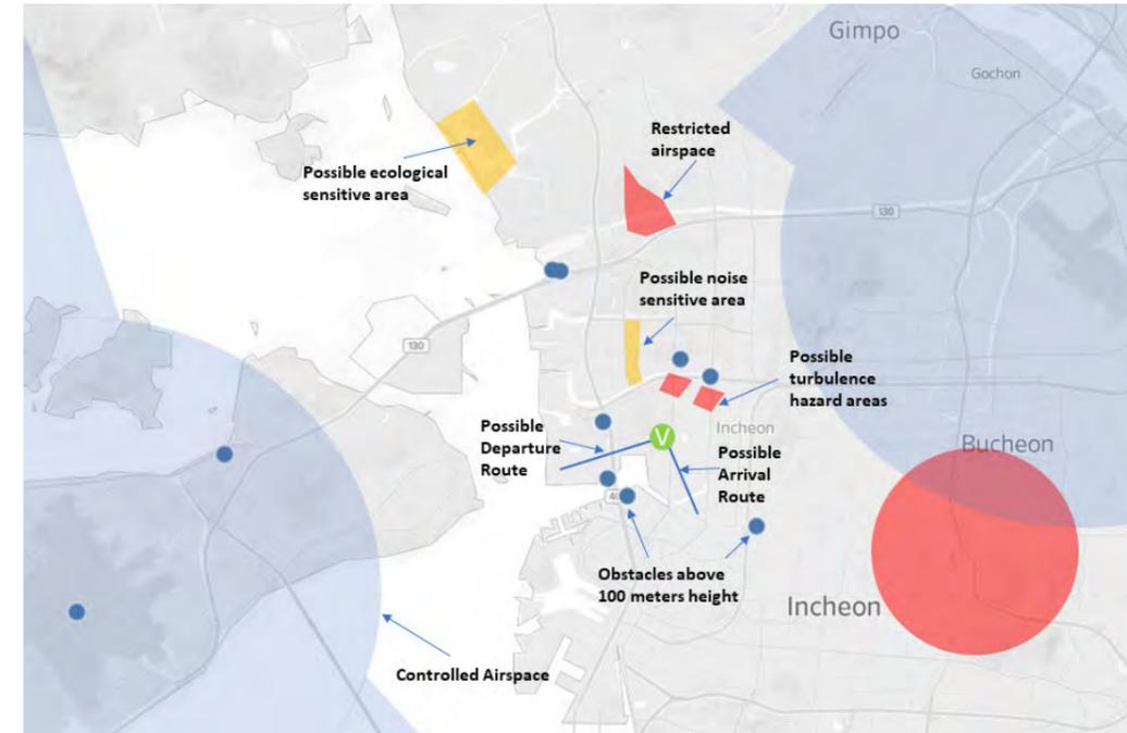
Considerations in vertiport flight procedure planning (This is a notional example chart based on an initial high-level analysis considering factors contributing to the selection of vertiport location.)
