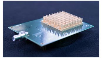
A 7-32 gigahertz additively manufactured (3D-printed) FUSE-onchip panel for satellite communication. FUSE's ability to move within the radio frequency spectrum boosts resilience. For more information about FUSE, visit mitre.org/WorkWithUs.
