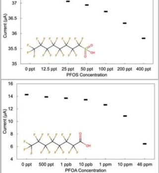
**Figure 1.** Left: A depiction of the impedence based detection of PFAS. The signal is reduced in the presence of PFAS by blocking access to the electrode. The reduction in signal is proportional to PFAS concentration. Right: Sensing curves for two common PFAS, PFOS and PFOA. Each can be detected from parts per trillion (ppt) to parts per million (ppm).
