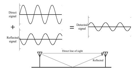
**Figure 1-15. Multipath interference**
