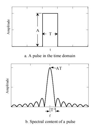
Figure 1-8. Frequency content of a rectangular pulse as a function of its dimensions
