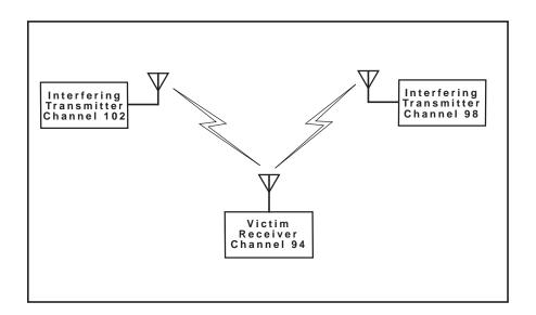
Figure 1-19. Intermodulation distortion at a receiver
