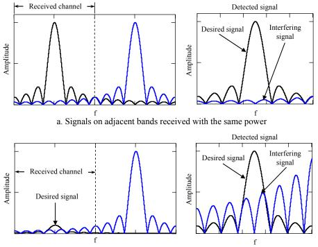
b. Signals on adjacent bands where the adjacent signal has a 10x power advantage
