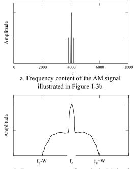
b. Frequency content of a typical AM signal where W is the bandwidth of the information
