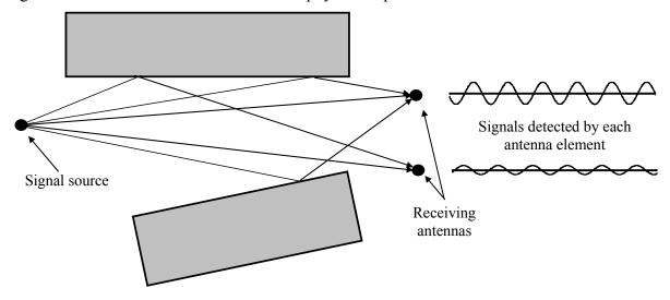
Figure 7-7. Differences in received signals caused by multipath arrival of signals at the receiving antennas
