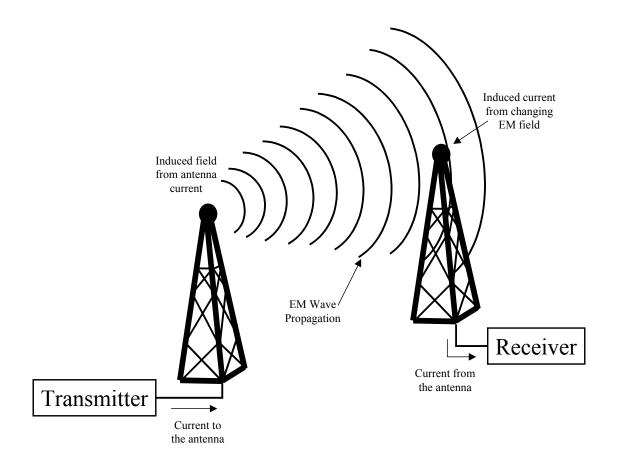
Figure 1-11. The transmission and reception of EM radiation
