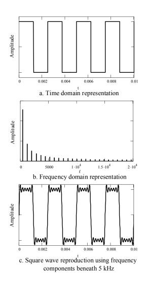
Figure 1-2. Representation of a 400 Hz square wave
