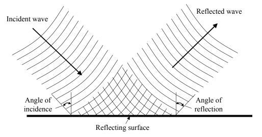
Figure 1-12. Reflection of an electromagnetic wave
