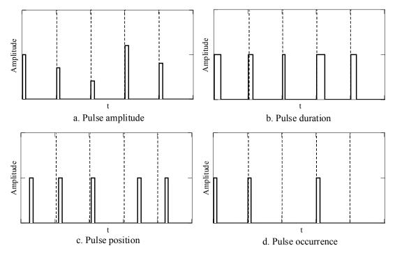
**Figure 1-6.** Pulse modulation methods
