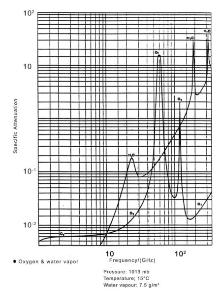
Figure 1-22. EM signal absorption by atmospheric gases
