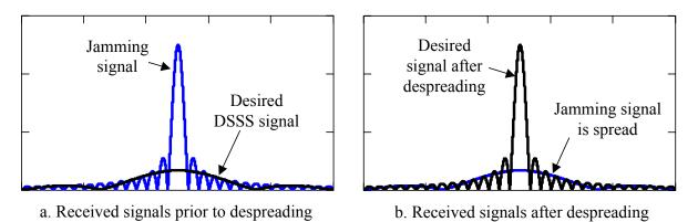
Figure 7-5. Anti-jam characteristics of DSSS
