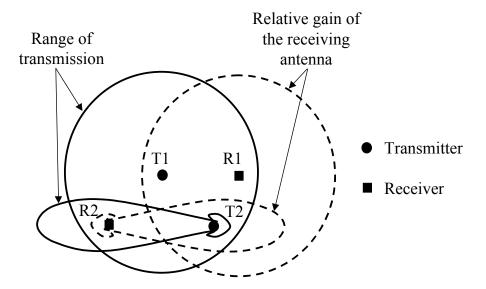
Figure 7-2. Comparison of omni-directional and directional antenna coverage.
