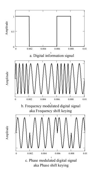
Figure 1-4. Example modulation of a digital signal
