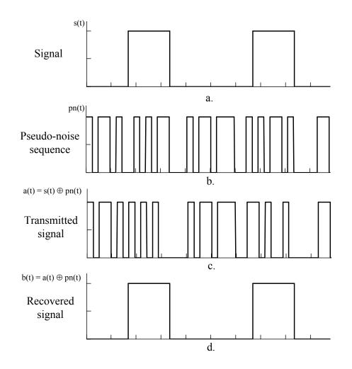
Figure 7-4. Example of Direct Sequence Spread Spectrum (DSSS)
