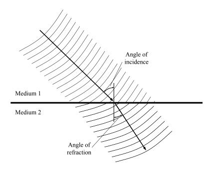
Figure 1-14. Wave refraction (propagation is slower in Medium 2 than in Medium 1)
