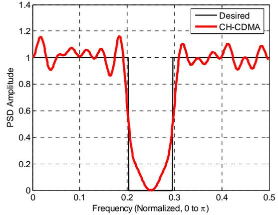
Figure 3: Bandstop-shaped PSD using length-32 WH codes.
