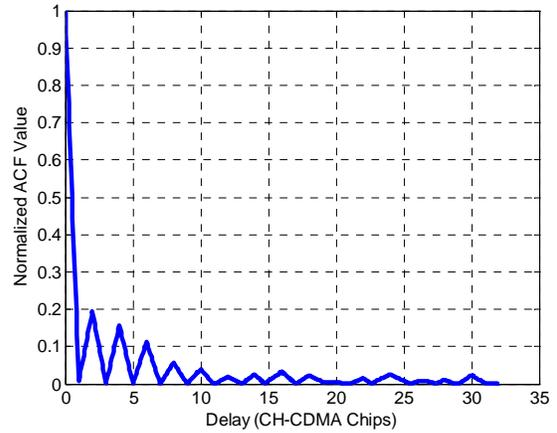
Figure 4: ACF of bandstop-shaped PSD using length-32 WH codes.
