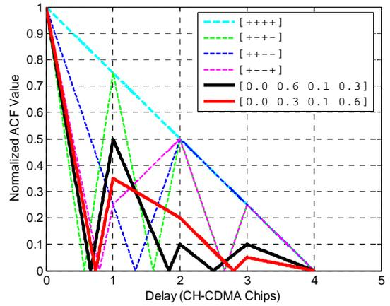
Figure 2: ACF's of the four length-4 WH codes and two CH-CDMA codes.
