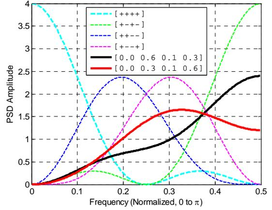
Figure 1: PSD's of the four length-4 WH codes and two CH-CDMA codes.
