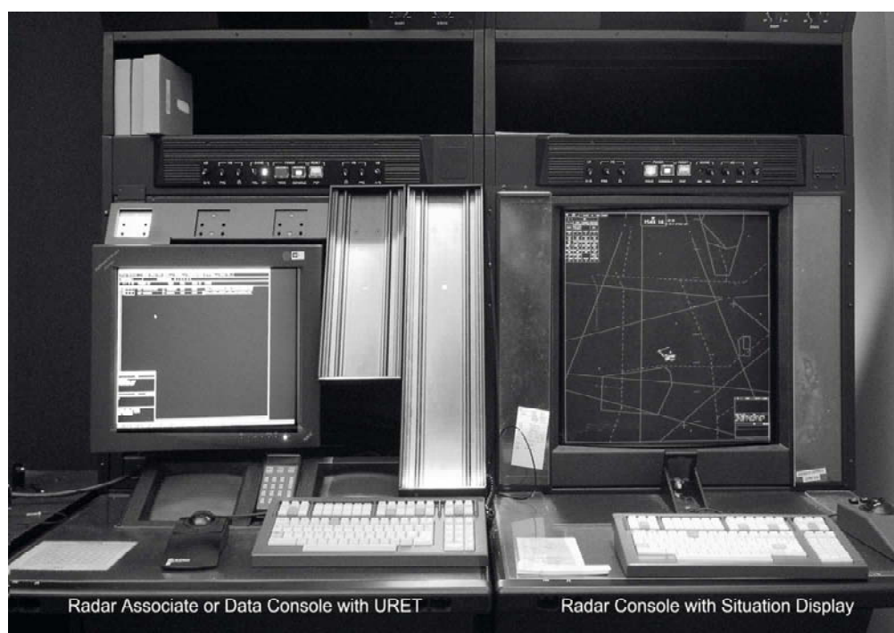
Figure 2 Radar Associate and Radar Consoles
