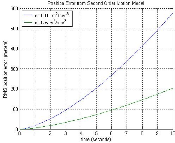
Figure 1. Position Errors from Second Order Random Motion Models
