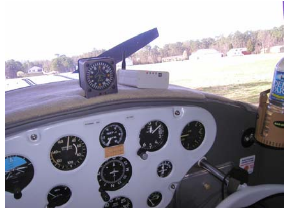
Figure 3. UAT Beacon radio on aircraft glare shield.
