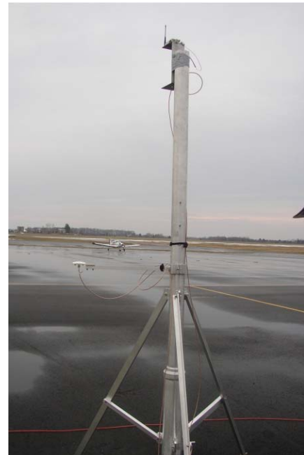
Figure 6. Emulate UAT Beacon radio on tripod.
