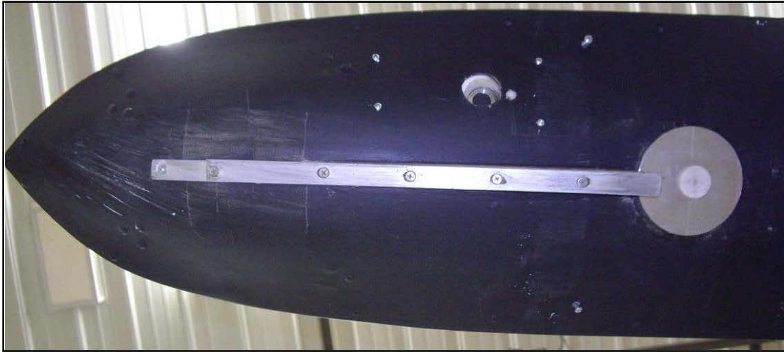
Figure 5 CDL Antenna Mounting and Landing Skid
