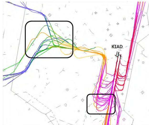
**Figure 1. Vectors for Arrival Spacing.** *This historic track data depicts RNAV arrival operations into Dulles International Airport. Note the dispersion of the tracks near within the highlight merge points.*
