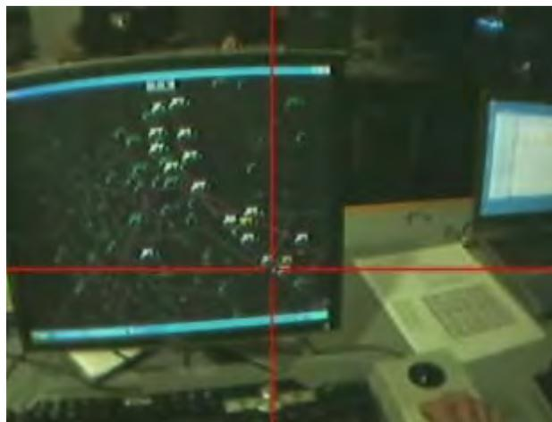
**Figure 8. Example Eye-Tracking Observation from RNAV with RPI Scenario.** The red line facilitates locating a fixation point for each ½ second observation.
