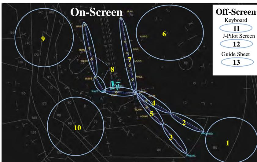
**Figure 7. Eye-tracking Areas of Interest.** Thirteen zones were established for fixation analysis of the South East feeder controller.
