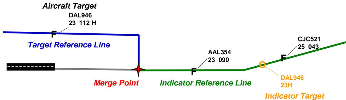
**Figure 2. Depiction of a Generic Relative Position Indicator (RPI) Application.** *The indicator target of the aircraft on the Target Reference Line is depicted the same distance away from merge point along the Indicator Reference Line, accounting for turn anticipation through the route segment transition.*
