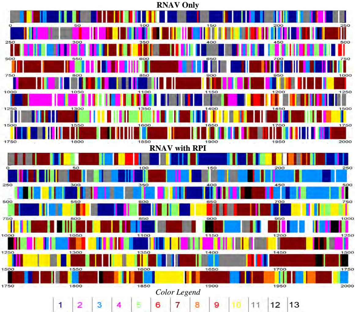
**Figure 9. Fixations in Areas of Interest for RNAV only and RNAV with RPI.** The plots present color-coded lines whose thickness indicate the number of 1/2 second observation (out of 2000) which fell with the area indicated in the color legend (mapped to Fig. 7). The white spaces correspond to “error”, which occurred when the eye-tracking equipment was unable to determine a fixation point.
