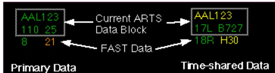
**Figure 11. Passive Final Approach Spacing Tool (FAST) Data Block [16].** The third line of the displayed data block contains the FAST advisory information. The green field is time shared between the pFAST relative sequence number to the runway and the pFAST runway assignment advisory. The second, colored data field is only used FAST.
