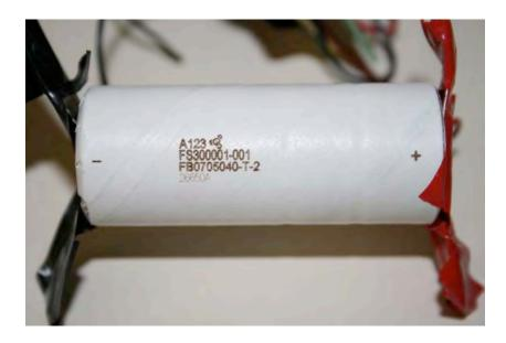
**Figure 3**. A123 Systems nanotechnology-enabled battery, with an LiFeO<sub>4</sub> cathode, used as the high-energy storage component in the NHPS. This battery is approximately 6.5 cm long.
