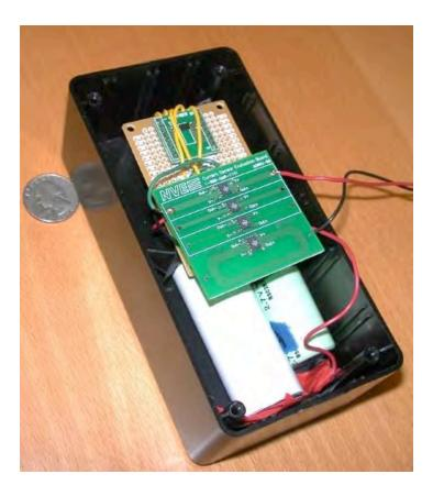
**Figure 6**. Initial laboratory prototype of nanotechnology-enabled portable power system that was assembled and tested in this work. A better packaged version of the system, with the control circuit breadboard replaced by an integrated circuit chip, would occupy only about 60 cm<sup>3</sup>.
