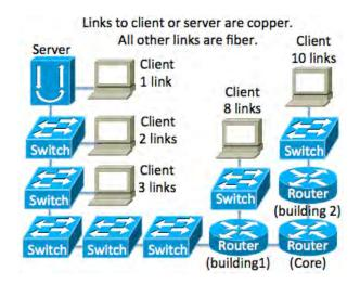
Figure 4. Network topology for timing experiments
