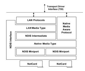
Figure 1. NDIS Architecture diagram from [12]
