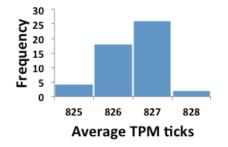
Figure 10. TPM tickstamp frequency distribution for 50 keys. STMicroelectronics TPM in Dell Optiplex 960.
