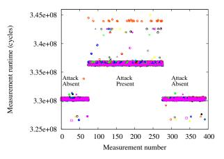
Figure 6. Rdtsc-computed runtime for 31 Dell Optiplex 960s. 2 second measurement frequency.
