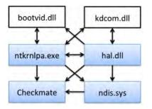
Figure 2. Checkmate kernel module dependencies
