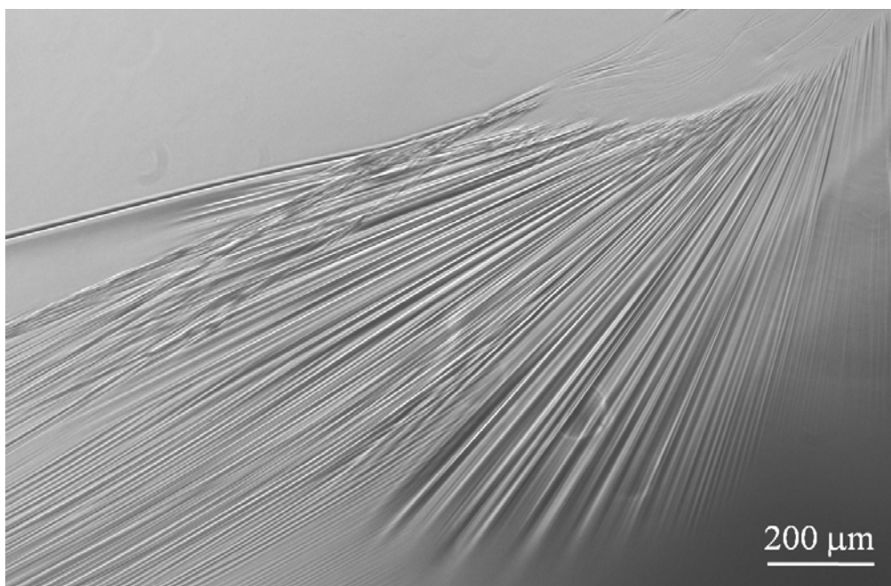
Figure 2. Stretch marks in a glycoprotein film lying at the interface between canola oil and an aqueous solution of chicken egg white glycoproteins, as photographed with an Olympus DP70 Digital Camera through a 10x lens using differential interference contrast (DIC) optics on an Olympus BX51/BX52 microscope.
