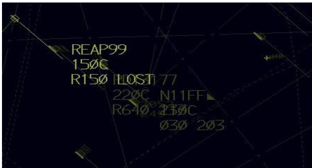
Figure 8. LOST Indicator on Controller Scope After Receiving Lost Link Activation via Data Comm from GCS
