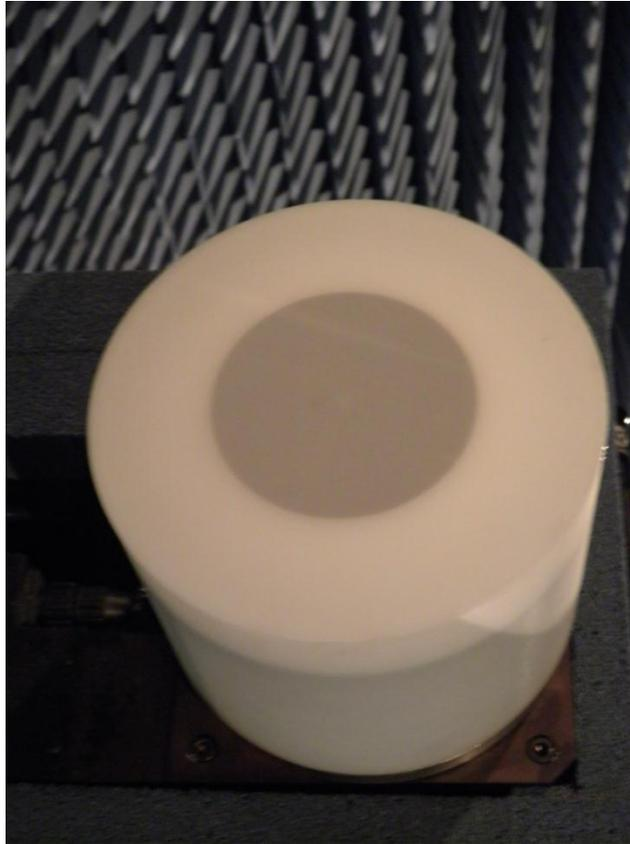
Figure 2.1-5. Radome placed over the Antenna and Mounting Fixture.
