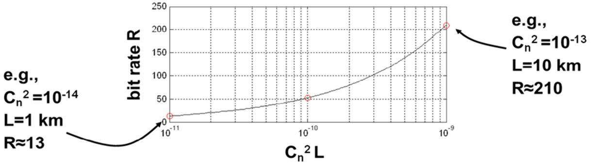
Fig. 16 Random bit rate versus product of  $C_n^2 L$  (simulation)
