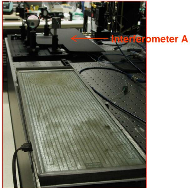
Fig. 7 Heater plate used to create simulated atmospheric turbulence
