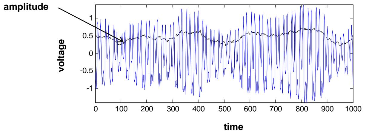
Fig. 10 Amplitude and dithered phase variations
