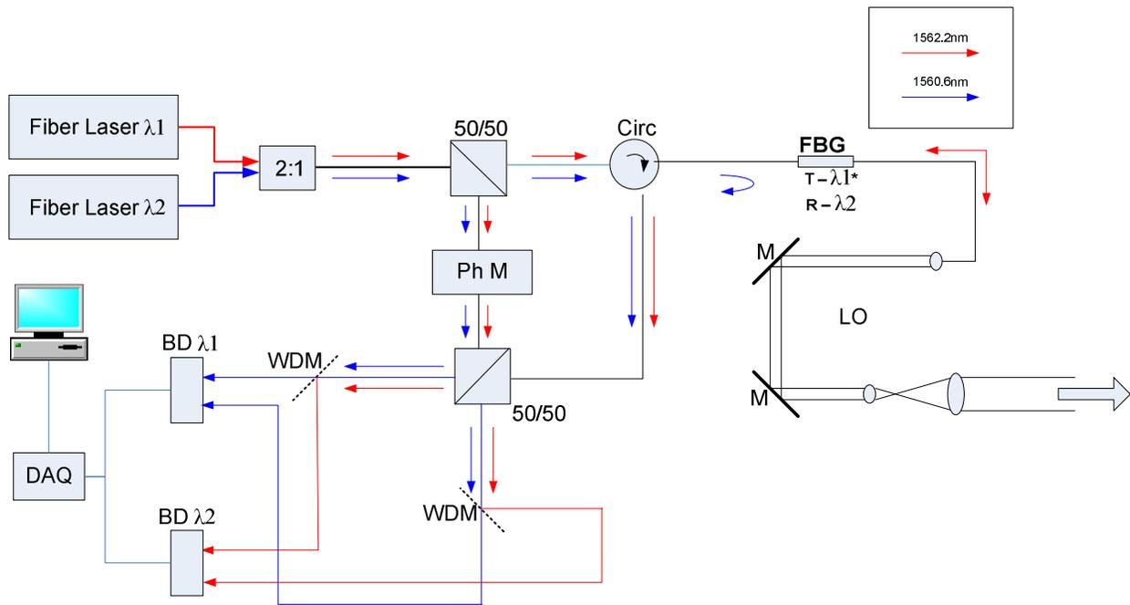
Fig. 5 COPIA terminal schematic. FBG = fiber Bragg grating, Ph M = phase modulator, WDM = wavelength division demultiplexer, BD = balanced detector, DAQ = data acquisition
