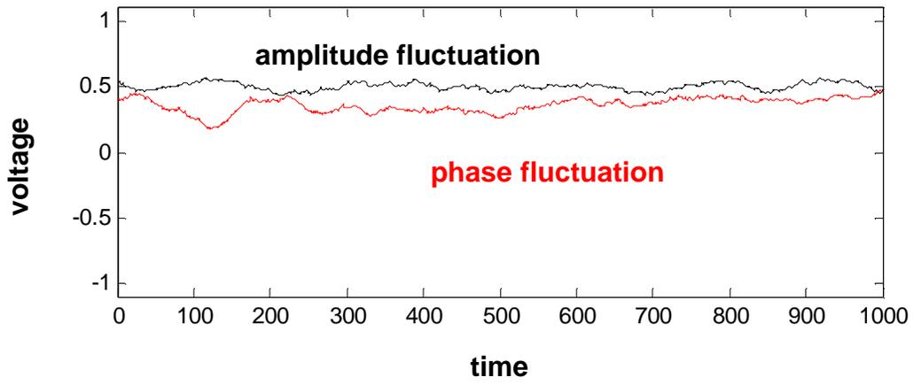
Fig. 9 Amplitude fluctuations may mask phase fluctuations
