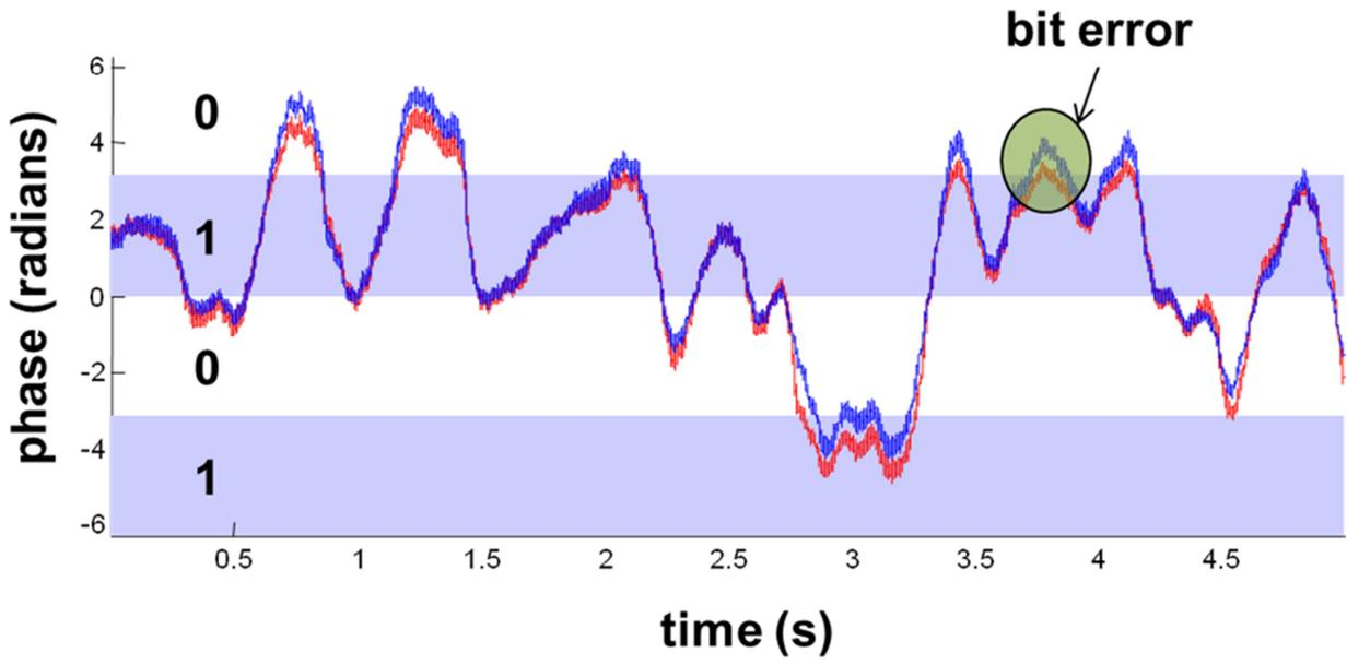
Fig. 12 Bit errors at inflection points of differential phase measurements
