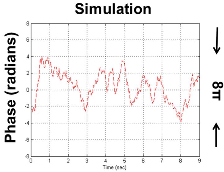
Fig. 15 Simulation of differential phase with laboratory parameter values (compare to the lab experimental measurements shown in Fig. 11)
