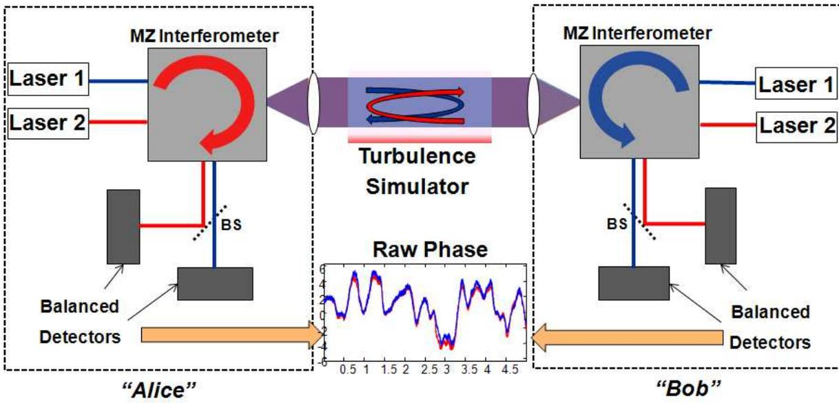
Fig. 4 Diagram of the COPIA optical system
