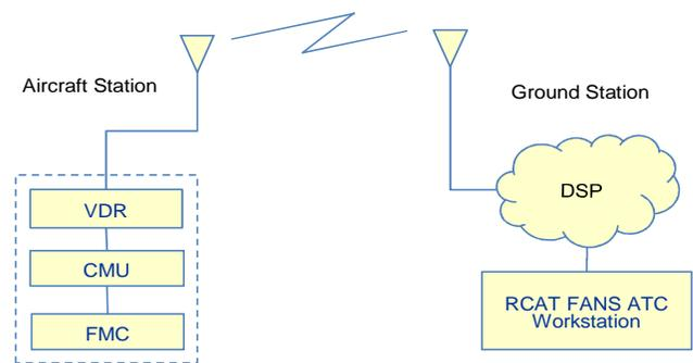
**Figure 4. RCTP Measurement Setup Diagram**
