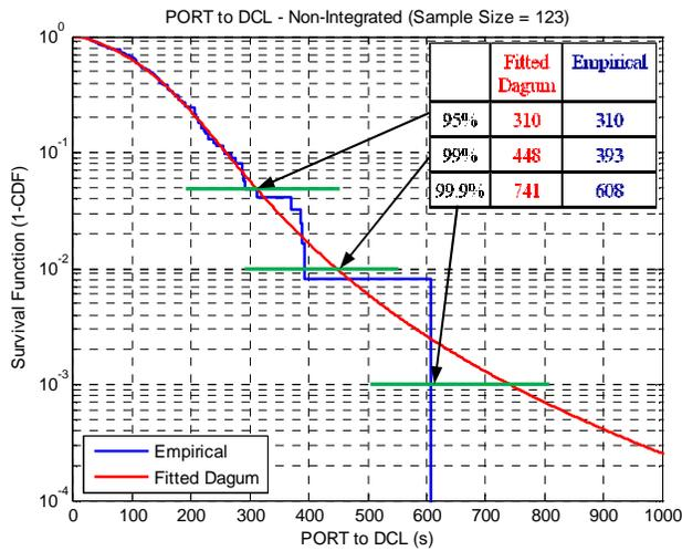
**Figure 8. DCL PORT Estimated Percentiles with Non-Integrated Implementation**
