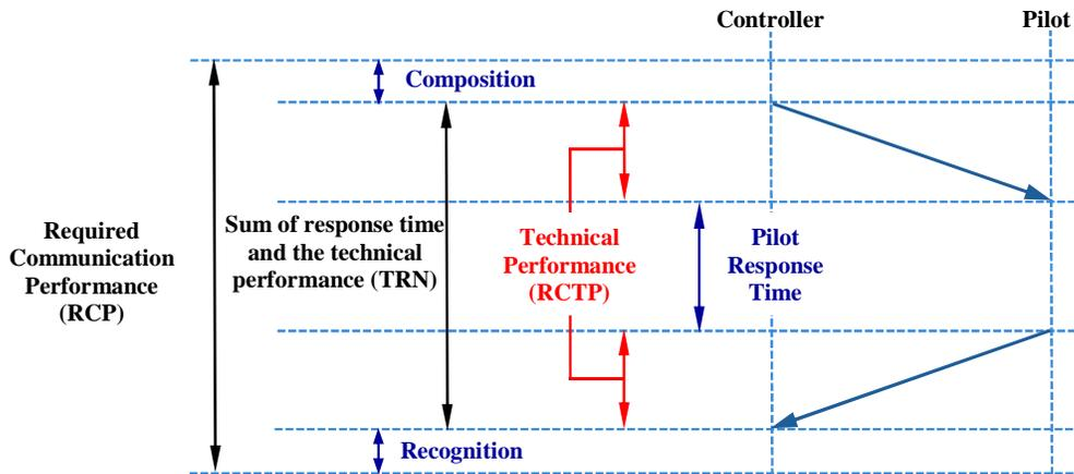
**Figure 3. Exchange Transaction Diagram**
