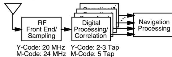
Figure 8. Receiver Architecture
