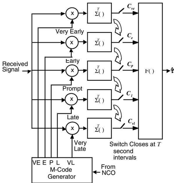
Figure 9. Code Tracking Loop Architecture for Very-Early/Very-Late Processing
