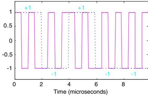
Figure 2. Example Segment of BOC(10,5) Baseband Signal (Solid Line), with Spreading Code Sequence +1, -1, +1, -1, -1 (Dashed Line)
