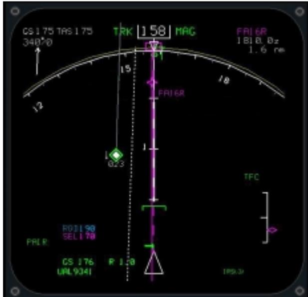
**Figure 4.** Navigation display- Paired approach engaged. Target position achieved.
