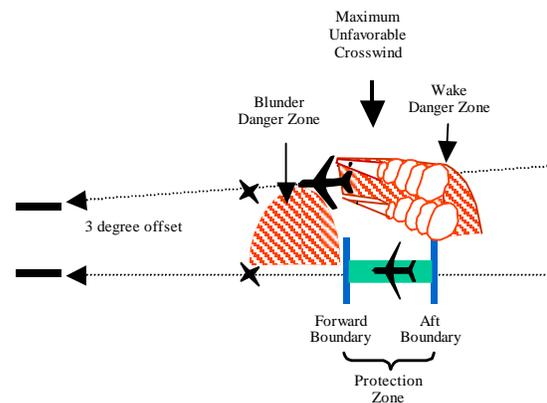
Figure 1. Paired approach concept plan view.
