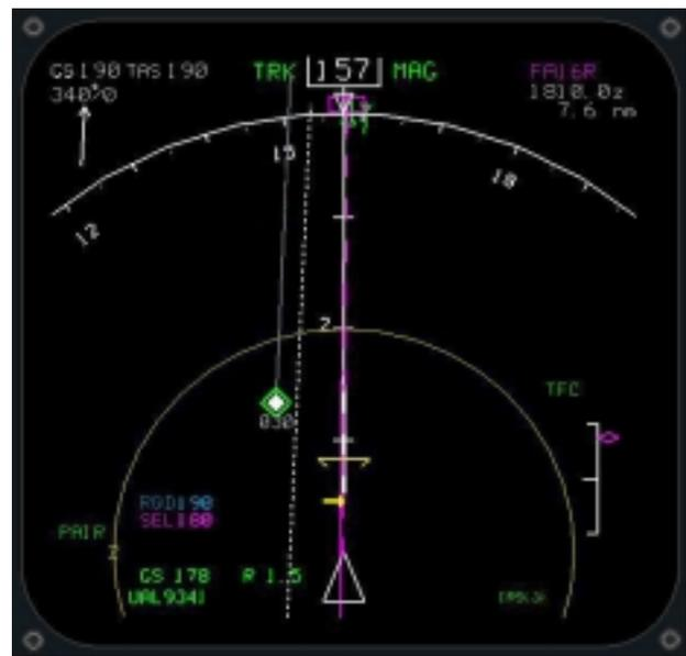
Figure 3. Navigation display- Paired approach engaged. Target position not achieved.
