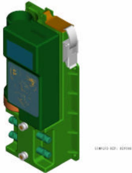
Figure 3: (U) JCAD Universal Mount with Detector Unit Attached
