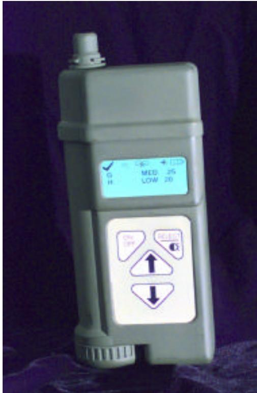
(U) The low level detection requirements are accomplished with the use of a pre-concentrator (PC). Figure 2 shows the detector unit with the PC attached. The PC is a
