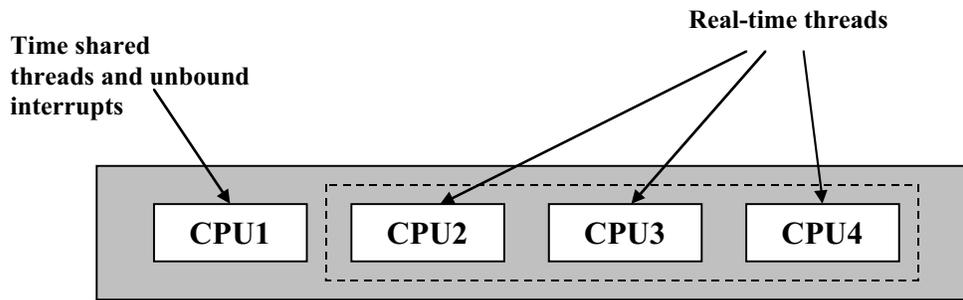
**Figure 2: Solaris Processor Binding and Control**
