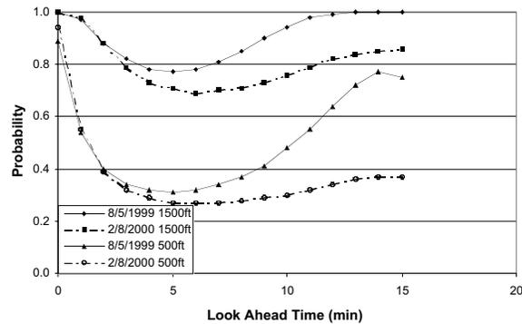
**Fig. 6 Vertical Prediction Accuracy During Descent**
