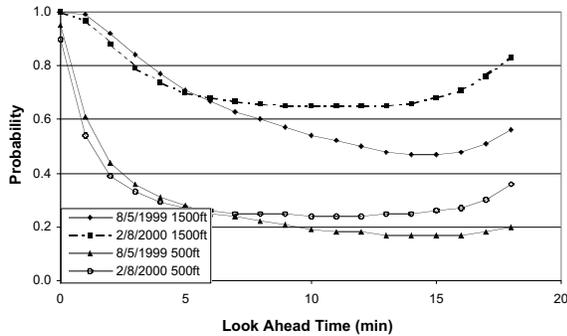
**Fig. 5 Vertical Prediction Accuracy During Climb**
