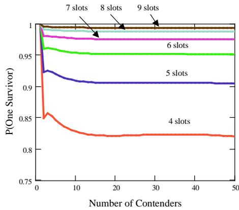
Figure 6. Contention resolution performance of different signaling designs
