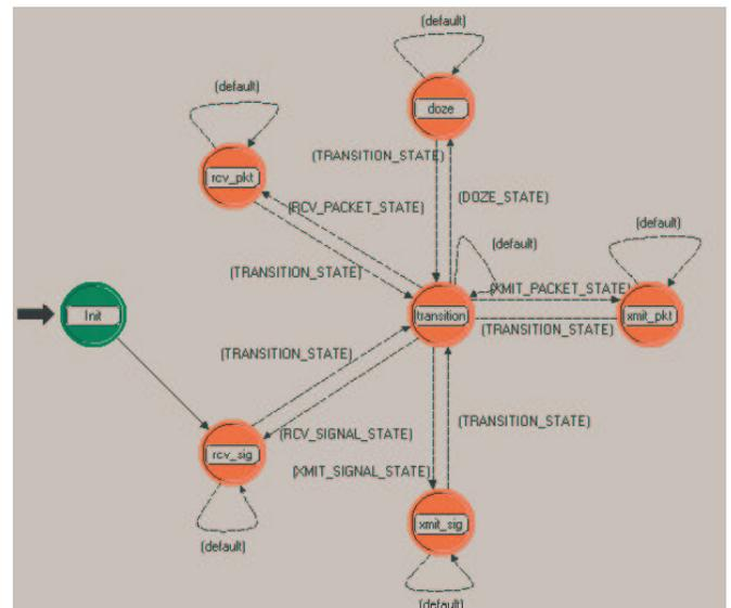
Figure 11. State diagram of the radio process
