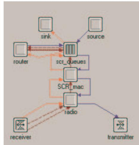
Figure 10. The SCR wireless node model
