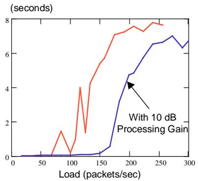
Figure 17. End-to-end delay
