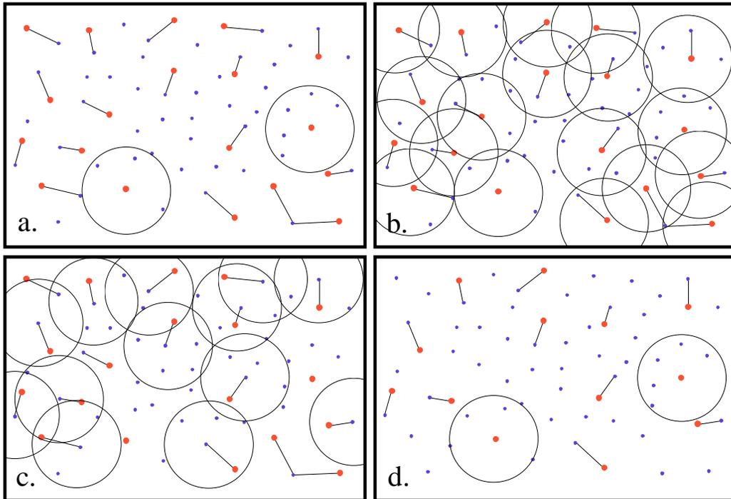
Figure 8. Example of the RTS-CTS handshake finalizing the set of nodes to exchange packets: Panel a illustrates the set of contenders that survived signaling and their intended destinations (circles indicate intended broadcasts). Panel b illustrates the contenders' simultaneous RTS transmissions. Panel c illustrates the destinations' simultaneous response of CTS packets. Panel d illustrates the winners of the contention.
