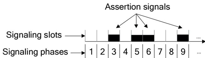
Figure 5. Collision Resolution Signaling using single slot phases
