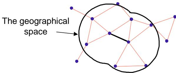
Figure 2. An example of a channel space required for a connection between two nodes. The extent of the channel space determines the membership of the distributed queue, in this case all nodes.
