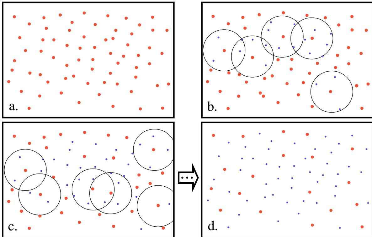
Figure 4. An example of the effect of Collision Resolution Signaling: All nodes start off as contenders (large dots) in Panel a. Then, through a series of signals, two sets of which are illustrated in Panels b and c, a final subset of contenders is selected in Panel d. The large circles represent the range of the signals. The small dots represent nodes that have deferred from contending.
