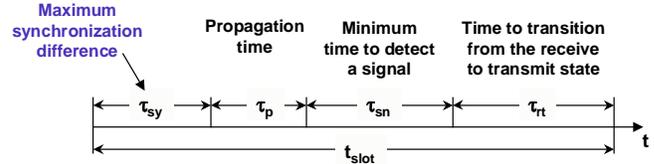
b. Factors that affect the sizing of a signaling slot in SCR
