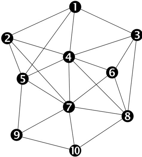
Figure 1. An example of link interdependence in wireless networks: When the directed connection from 4 to 7 is used, no other directed connection may be used.
