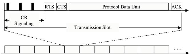
Figure 3. The Synchronous Collision Resolution Protocol
