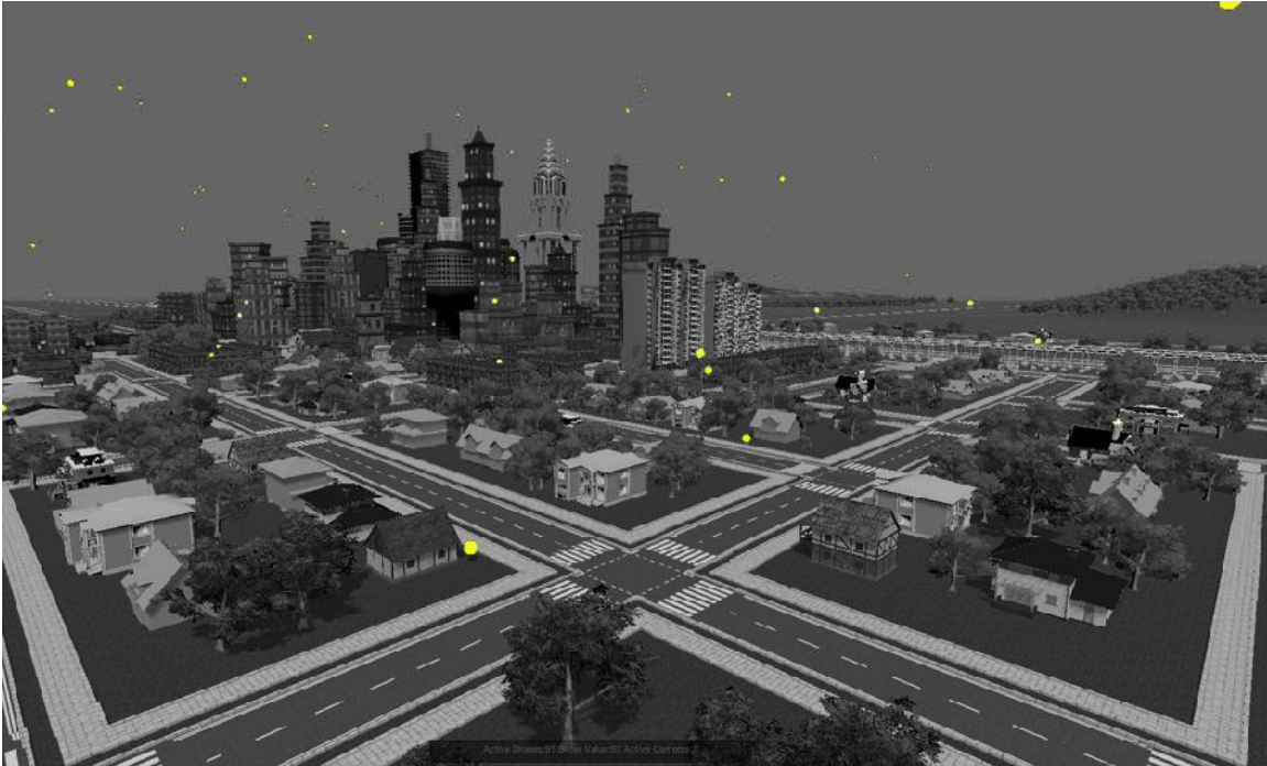
Figure 4: Simulation of Future High Density SUAS Operations (90 drones per square mile) (SUASs Enveloped in 8ft Diameter Yellow Spheres for Better Visibility)
