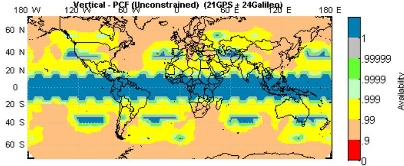
**Figure 3. LPV-200 Availability of Vertical Integrity for the New Method Assuming an Unconstrained Consistent Fault (21 GPS and 24 Galileo)**
