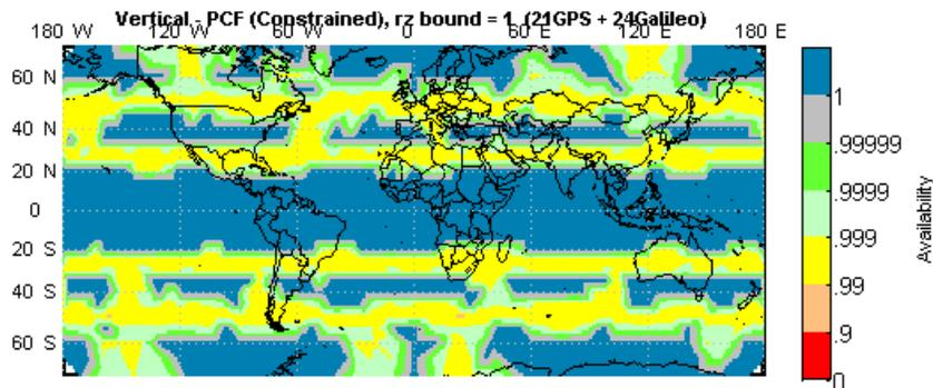
**Figure 4. LPV-200 Availability of Vertical Integrity for the New Method Assuming a Consistent Fault Constrained with  $|r_U|$  Bound = 1 (21 GPS and 24 Galileo)**
