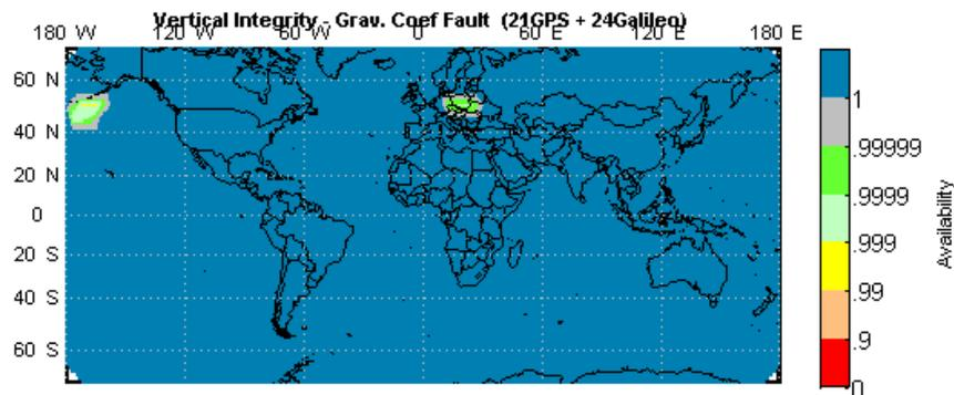
**Figure 6. LPV-200 Availability of Vertical Integrity for the New Method Assuming Presence of an Erroneous Earth's Gravitational Constant (21 GPS and 24 Galileo)**
