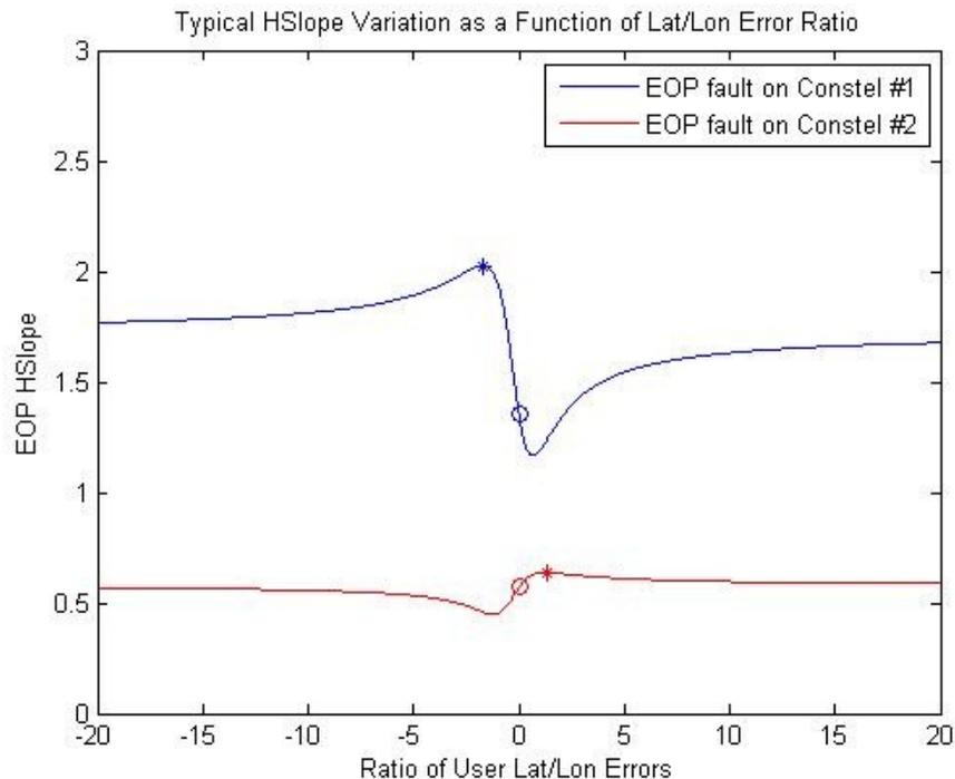
**Figure 1. Typical HSlope Variation for the New Method Assuming an EOP Fault as a Function of the Ratio of  $b_N/b_E$**
