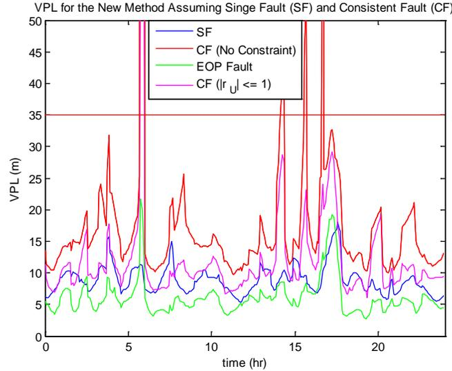
**Figure 5. Typical VPL Variation under Different Fault Assumptions**
