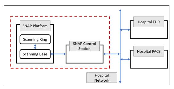
Figure 18: Example First Pass, High-Level DFD for the SNAP System. Only Major Hardware Components Are Outlined.
