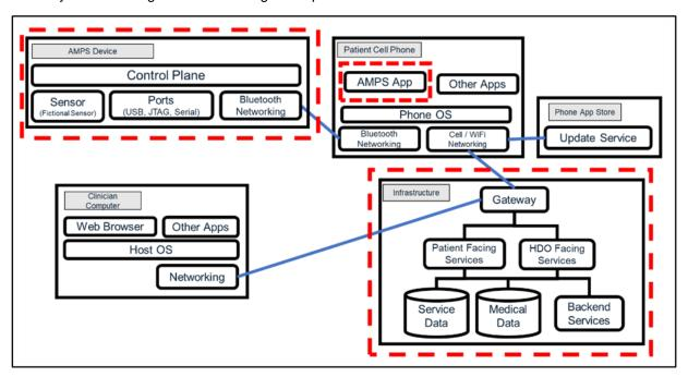
Figure 3: Example High-Level Trust Boundaries of the AMPS Device DFD
