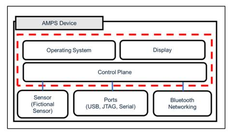
Figure 4: Example Device Trust Boundary
