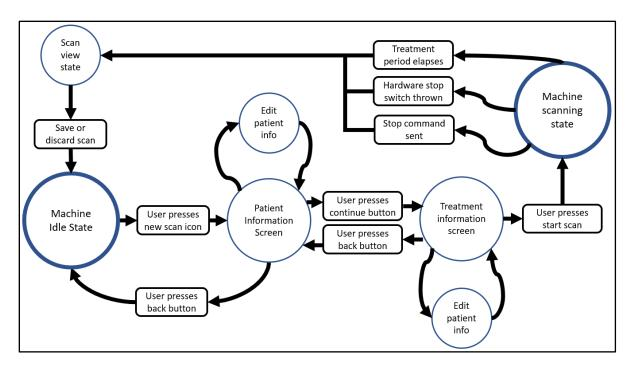
Figure 20: State Diagram for Initiating a SNAP Scan
