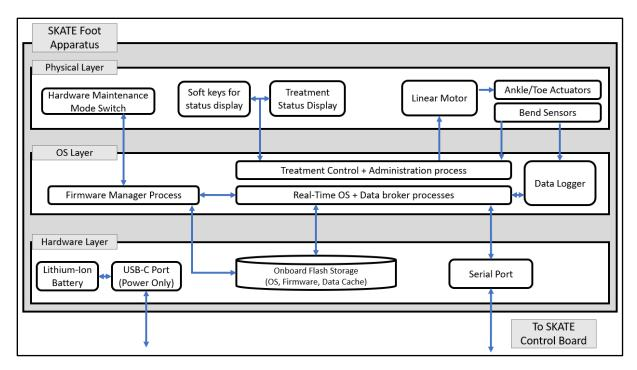
Figure 26: Lower Level DFD for the SKATE Foot Apparatus
