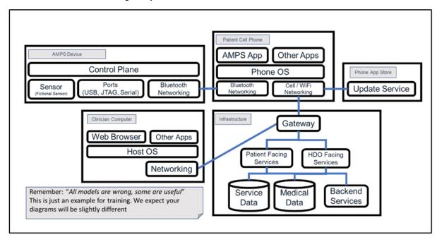
Figure 2: Example Mid-Level DFD for the AMPS Device (No Trust Boundaries)
