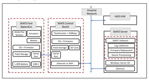
Figure 25: Data Flow Diagram for the SKATE System
