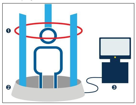
Figure 17: Diagram of the SNAP System. 1) The SNAP Scanning Ring. 2) The SNAP Scanning Base. 3) The SNAP Control Station.
