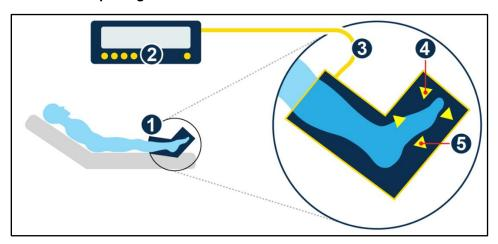
Figure 24: Picture of the SKATE device. The large circle provides a zoomed in version of the SKATE foot apparatus. 1) The SKATE foot apparatus. 2) The SKATE Control Board. 3) Connection between the foot apparatus and control board. 4) Motor and bend sensors for actuating the toe. 5) Motor and bend sensors for actuating the ankle.
