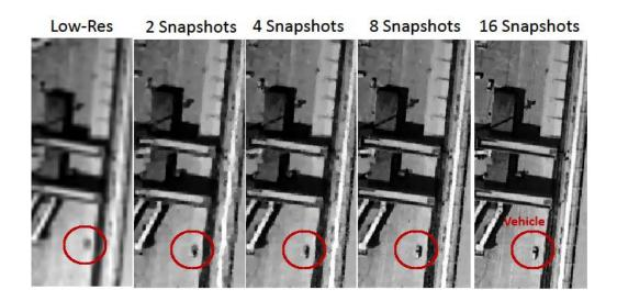
Figure 6: In this example, the object is an overhead photograph of the Zurich airport (terminal B) taken with Quickbird sensor via Google Earth. The ability to discriminate the vehicle (highlighted in the circle) improves as the number of snapshots increases.
