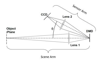
Figure 1: Diagram illustrating the experimental setup used to acquire ARCSI data. Lens 1 forms an image of the object plane on the DMD which is spatially coded with a binary pattern. Lens 2 then forms an image of the object plane multiplied by the binary pattern. Note that the figure is not to scale.
