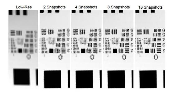
Figure 4: An example of images reconstructed from 2 - 16 snapshots using the approach described in Sect. 2. The image on the left represents a single down sampled acquired with all mirrors on and then binning the detector.
