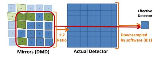
Figure 2: Sensor schematic showing the relative magnification between DMD and detector plane (1:2) and then the software down-sampling operation effectively making the compression ratio from DMD to effective detector as 16:1. This configuration allows the study of various ratios of mirrors to detector elements.
