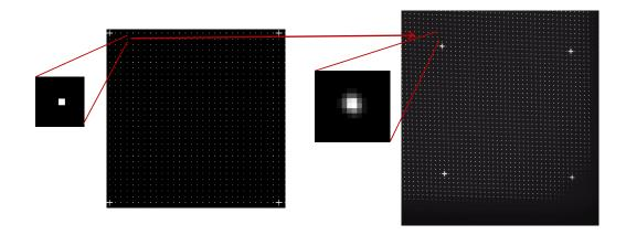
Figure 3: One frame of a typical ARCSI calibration. The left image is the input to the DMD while the right image is the response on the detector. The zoom-in shows the size of the psf. Matching the pixel on the left with a patch on the right allows us to build a precise linear model for the camera.
