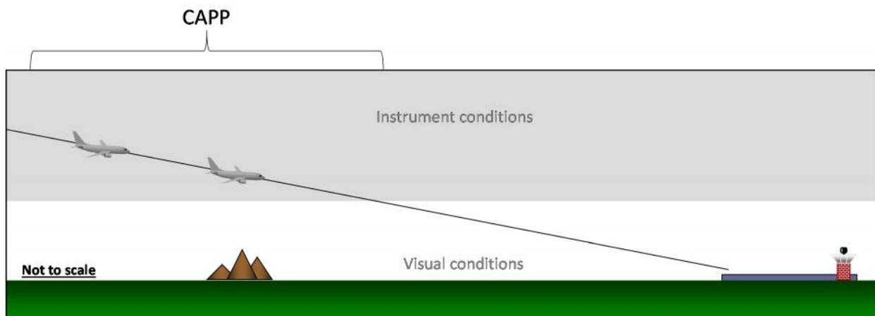
**Figure 4-6. Profile View of the CAPP Phase of the Approach**
