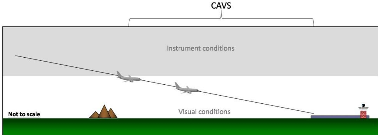
**Figure 4-7. Profile View of the CAVS Phase of the Approach**
