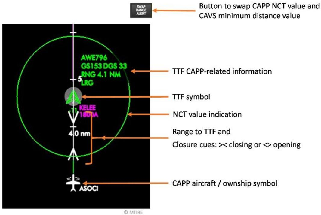
**Figure 3-7. CDTI Inset Showing CAPP Display Elements**
