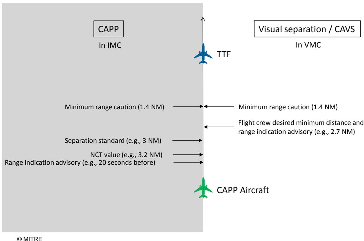
**Figure 2-3. CAPP versus CAVS spacing and alerting**
