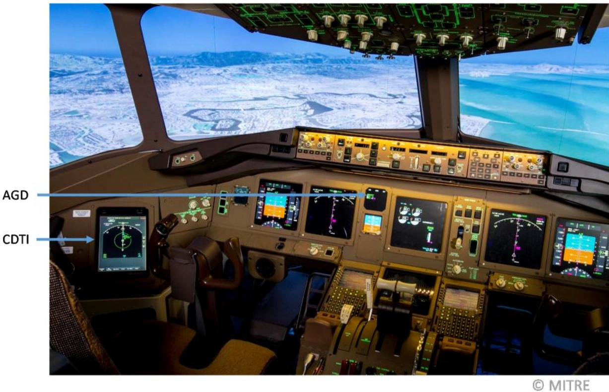
**Figure 3-4. CDTI and AGD Location in Flight Deck Simulator**
