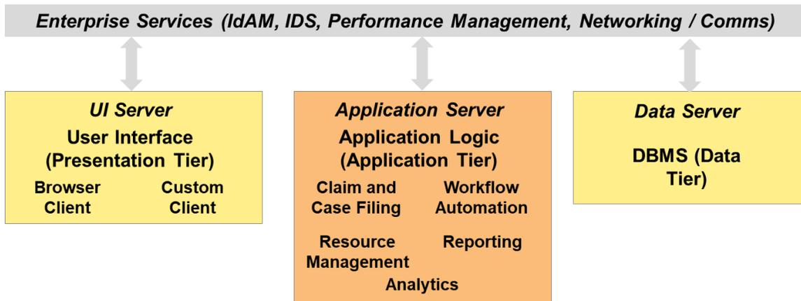
**Figure 7. Three-Tier Architecture for Notional CRM Application**
