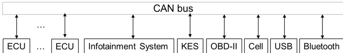
**Figure 9. Vehicle Architecture**
