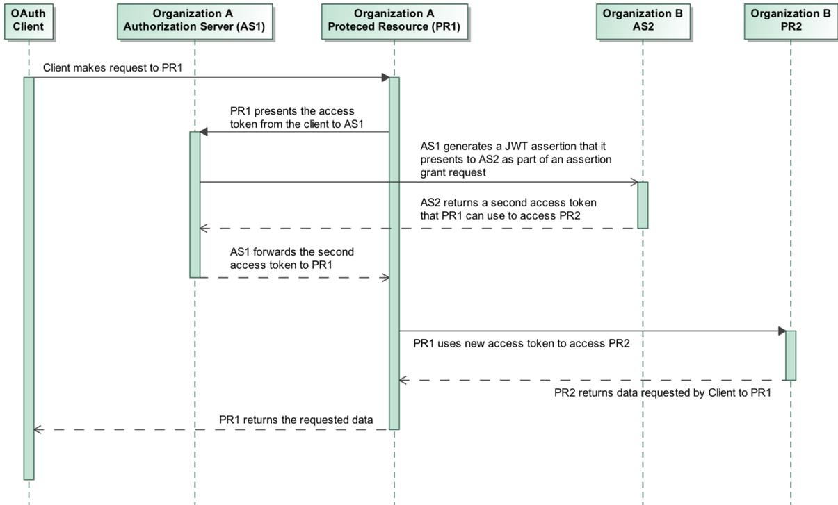
**Figure 10: Option 3b for Token and Identity Chaining in a Multiple ICAM Ecosystem**
