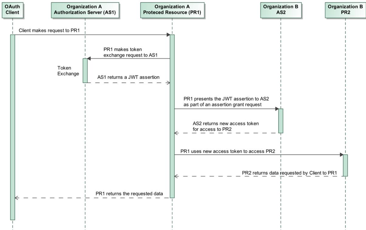
Figure 8: Option 3a for Token and Identity Chaining in a Multiple ICAM Ecosystem
