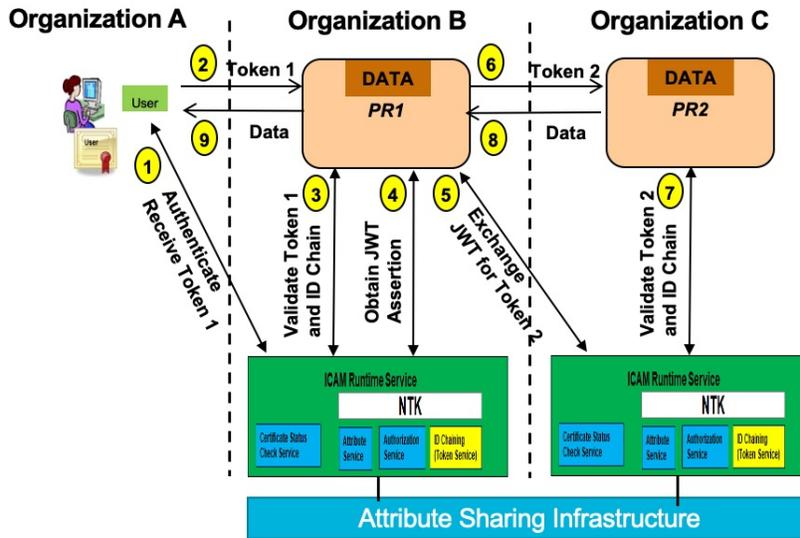
Figure 7: High-level view of token chaining in a multiple ICAM ecosystem using Option 3a
