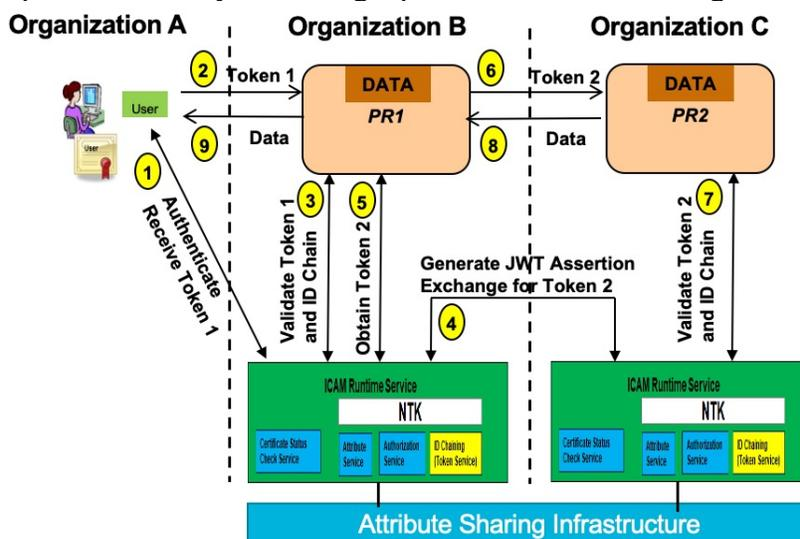
**Figure 9: High-level view of token chaining in a multiple ICAM ecosystem using Option 3b**
