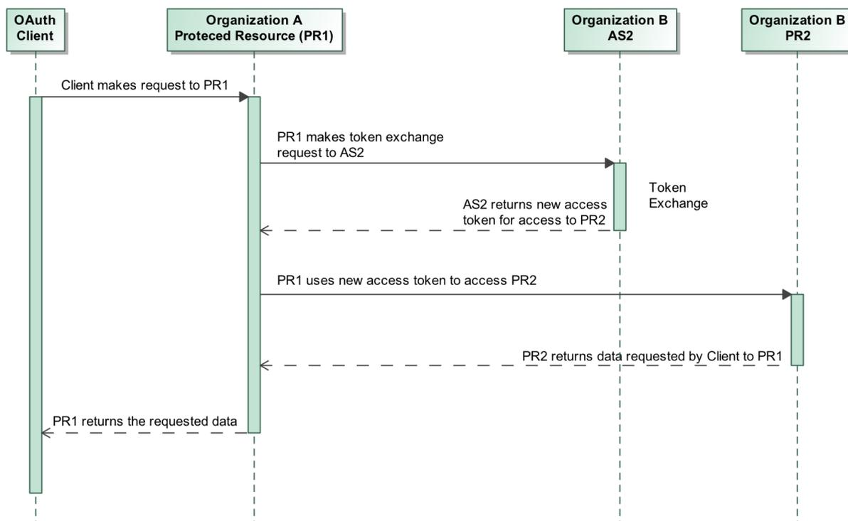
**Figure 6: Option 2 for Token and Identity Chaining in a Multiple ICAM Ecosystem**
